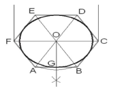
**Q.11.** A thin horizontal hexagonal plate of 15 mm sides is inclined at 45° to the H.P. and perpendicular to V.P. two of its parallel edges is parallel to V.P. Draw the projections of the plate.
